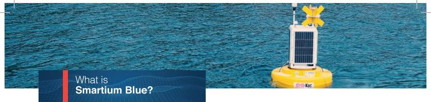
Smartium Blue is a measurement & observation system which continuously monitors the oceanographic and atmospheric environment, provides data to users via web-based applications, informs and warns them if the preset thresholds are exceeded.
